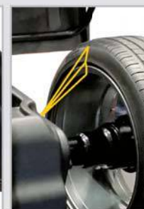
GAR334 LASERHEAD Internal and external laser blade shows precise 12 o'clock position in dynamic mode.
