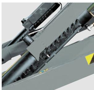
Mechanical locking device with automatic engagement and pneumatic release, ensuring maximum safety when lift is raised.
