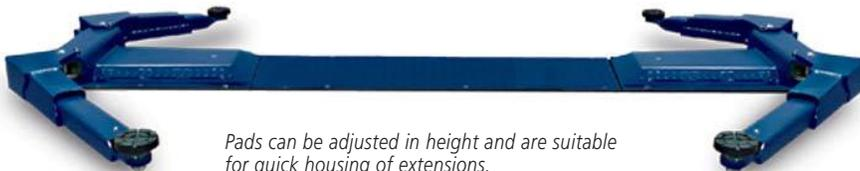
Pads can be adjusted in height and are suitable for quick housing of extensions.
