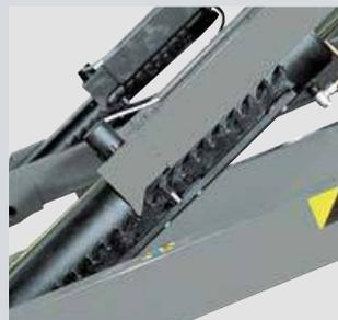
Mechanical locking device with automatic engagement and pneumatic release, ensuring maximum safety when lift is rised.
