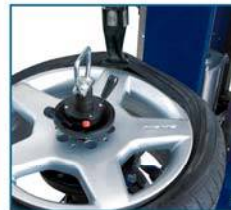
Levering on the rim, the tool pulls up the bead, minimizing tire stress
