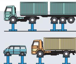
Modular electrical systems enable alterations to be made to configuration (e. g. passing 4 to 6 to 8 columns, or creating two sets of 4 columns by splitting a set of 8).
