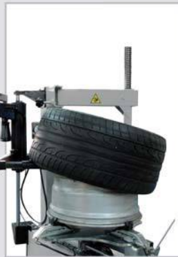
PLUS915A for G7246 PLUS91N for G7240 Pneumatic helper with rotating arm
