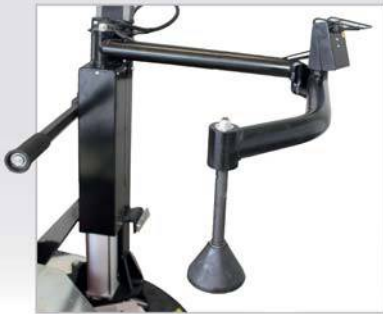
PLUS83H Air-driven helper with rotating arm
