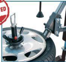
The tool enters between bead and rim
