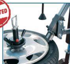
The tool enters between bead and rim
