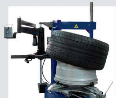
DEMOUNTING (lower bead)
