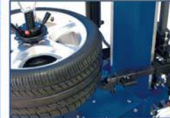
Levering on the rim, the tool pulls up the bead, minimizing tire stress
